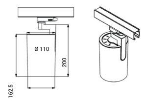
Ray Mini uses the possibilities created by new technology. The LED driver is mounted inside the luminare body. This gives us a slim design combined with a powerful lightoutput that can be easily adjusted in all directions to meet all needs. Ray Mini can be tilted 90 degrees and rotated 350 degrees its own axis. To create further opportunities to play with light you can mount a diffuser on the luminaire, this can be ordered separately.
