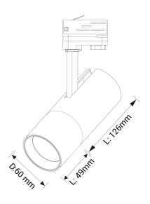
The Cylinder 60 has the LED driver included in the lamp head and is available for use in 1-circuit and 3-circuit tracks, both models are available with a Dim to Warm option. It can be tilted 90 degrees and rotated 350 degrees on its own axis and comes with a variety of accessories.
