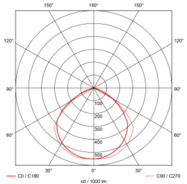
Sign Today Mini comes with a 105x90° beam angle. The luminaire is manufactured in die cast aluminum. Sign Today has built-in LED driver and comes with 1m cable.
