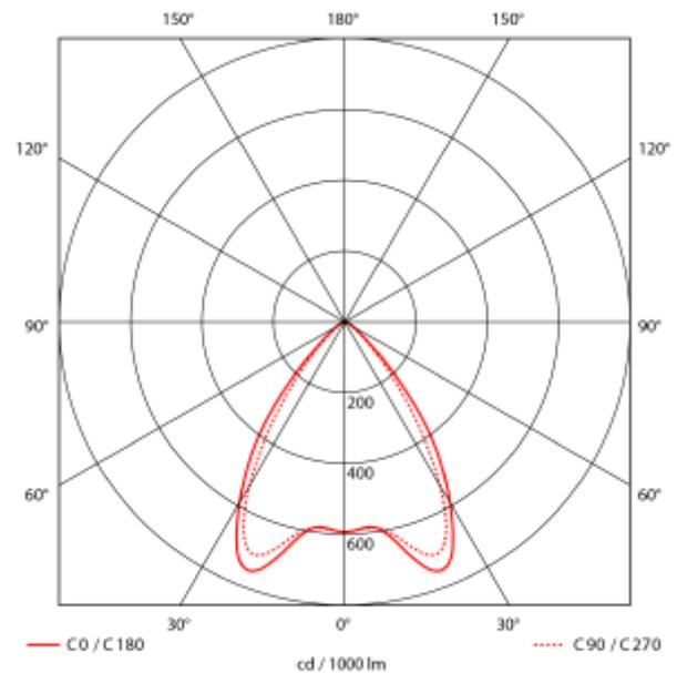
Bladeline Z is a highly efficient LED luminaire with up to 179lm/w. Due to fact that it may be installed surface mounted on the ceiling or on electrical tracks makes it highly flexible. Can be opened without using tools and it has the electric connectors on quick fit clamps. The Bladeline Z is made from galvanized steel with medium or wide beam (75° and 90°) optic in 42W or 75W versions.
