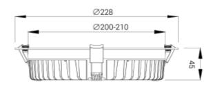
Antares downlight have high lumen output and PMMA diffuser with even light distribusion. Comes with a switch option between 3000K(default), 4000K and 5700K. All data is based on 4000K.
