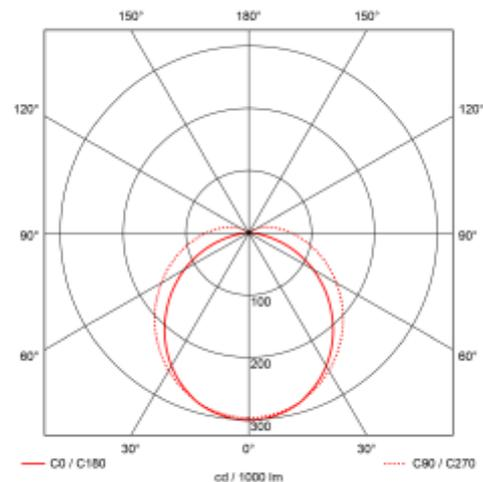
Stream C is a sealed industrial light fixture for ceiling surface mounting or pending down with wires, indoor and outdoor. The Stream is classified in accordance with IP65. The light fixture is made from robust fiber glass and is equipped with a milky white (opal) diffuser w/stripe. The Stream is prepared for cable 5×2,5mm<sup>2</sup> wiring through for an efficient installation.
