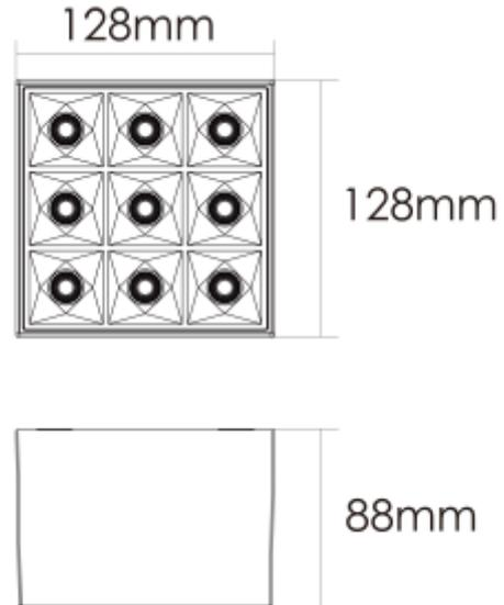
Phoenix Downlight has the latest LED technology, with micro reflector and anti-glare cover it reaches UGR17. With 35° beam angle and perfect light cutoff it's the ideal downlight for office, hotel, staircase, and corridors. Delivered with phasecut driver.
