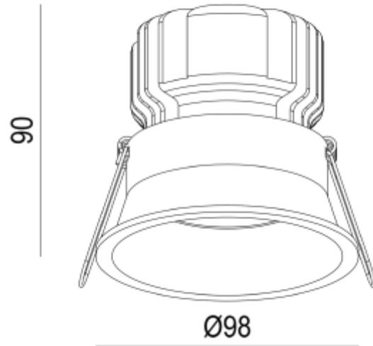
Ceto Fixed is a downlight with 15W effect and secluded light source. 36° beam angle and IP44 certified. Ceto Fixed is the natural choice if you are looking for an exclusive expression that provides a comfortable and good light. Dimmable phase-cut driver included.
