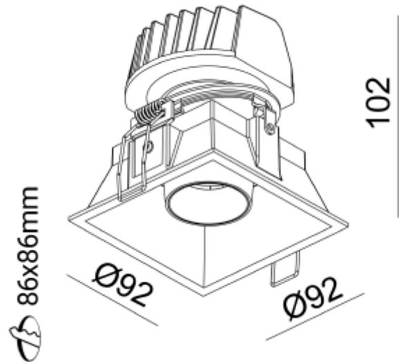
Make is a square downlight in single version that comes with Dim 2 Warm function. The color temperature (K) can be adjusted between 3000K and 1900K through dimming. Rotatable 360° and tiltable 20°. Driver is not included and sold separately. See accessories for recommended drivers.
