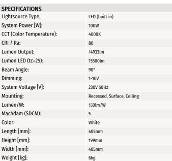
Petrol is a high luminous efficacy luminaire ideal for gas station as a retrofit or new installation. Delivered with 4000K in two versions. 100W and 150W with up to 150lm/w. Suitable for garage/gas station, warehouse, industrial facility, exhibition center and shopping mall. Surface mount kit are bought seperately.
