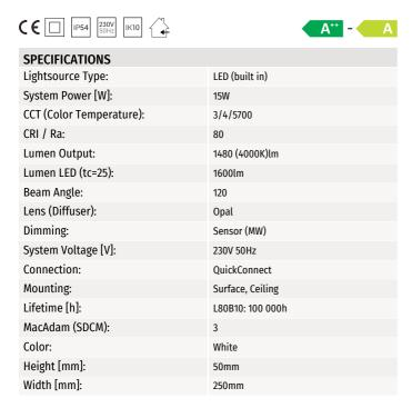
Pollux is a surface mounted ceiling light that adopts high lumen SMD LED, fire-rated PC diffuser with even light output. IP54 waterproof structural design, it s an ideal replacement for wet locations. Comes with a microwave sensor with various options.
