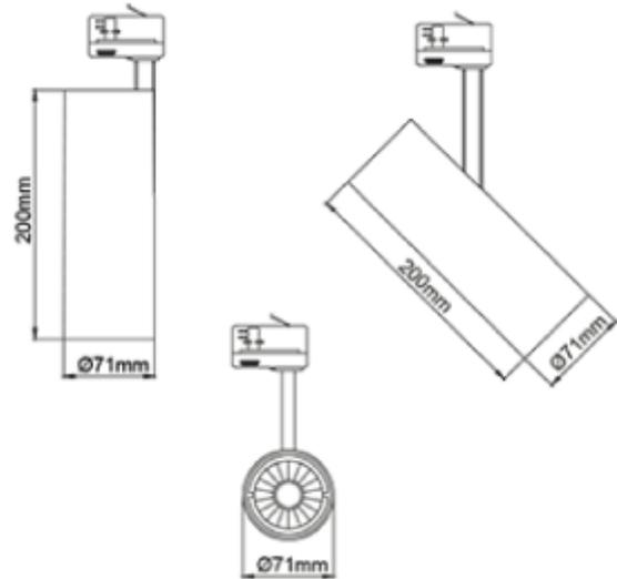
The Silindir uses the possibilities created by new technology. The LED driver is mounted inside the luminaire body. This gives us a slim design combined with a powerful light output that can be easily adjusted in all directions to meet all needs. Cylinder can be tilted 90 degrees and rotated 350 degrees its own axis.
