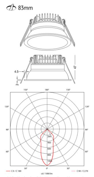
Ceto Mini fixed is a low downlight with 7W effect. With recessed light source, low blending, CRI95 and 36° beam angle, this is the natural choice where you want to create an exclusive and comfortable lighting. Phase-cut driver included.
