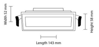
IP65 version of the popular Cold -series. With its rectangular shape and recessed light source, Cold provides a unique decorative design. Se accessories for recommended driver. Cut-out 130x36mm.
