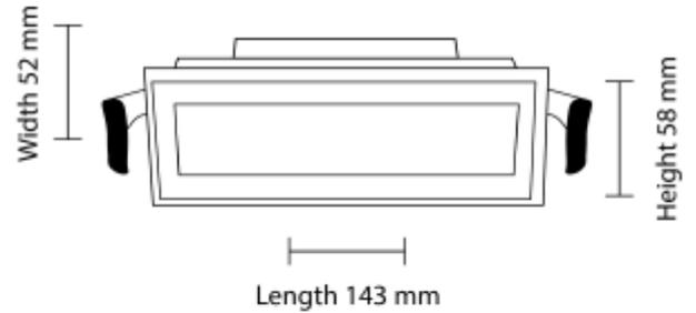
IP65 version of the popular Cold -series. With its rectangular shape and recessed light source, Cold provides a unique decorative design. Se accessories for recommended driver. Cut-out 130x36mm.
