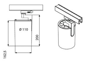
Ray Mini uses the possibilities created by new technology. The LED driver is mounted inside the luminare body. This gives us a slim design combined with a powerful lightoutput that can be easily adjusted in all directions to meet all needs. Ray Mini can be tilted 90 degrees and rotated 350 degrees its own axis. To create further opportunities to play with light you can mount a diffuser on the luminaire, this can be ordered separately.
