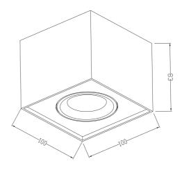
Cobra 360° Rotatable Surface is a flexible surface mounted downlight developed from our vast experience with earlier models. The 360° Rotatable light head makes it possible to tilt the light beam up to 25 degrees in all directions.
