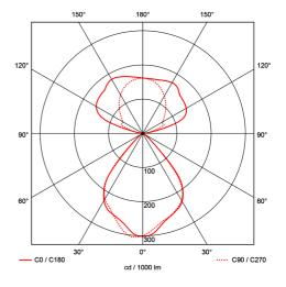
The Phoenix is a linear LED luminaire with up- and down light for pending down in indoor areas. The light distribution is 2000 lumen upwards with a 140° reflector and 2000 lumens downwards with a 80° reflector. It is made from durable aluminium for easy care. The color temperature is 3000 Kelvin and the reflectors secures a pleasant light. 3m wire.
