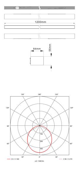
Ledline is a modern linear LED system for seamless lighting. It is based on modular chassis details allowing for seamless extensions through both straight connectors, 90 degrees corners and X-crosses. This allows light designers to make tailor fit lighting systems in an easy manner. The chassis details assure easy installation without failures.
