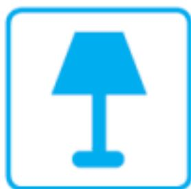
This luminaire contains built-in LED lamps.
