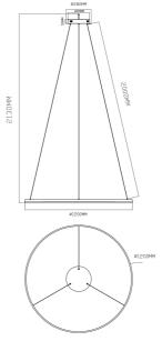
The Halo pendant range consists of 3 different sizes circular luminaires, they are made from aluminum, coated with a golden matt color. The opal surface covering the LEDs gives a very pleasant warm light in 3000 Kelvin. The length of the wires holding the circular luminaires can be adjusted on site making the Halo pendant very flexible for decorative purposes (wire length is 200cm).
