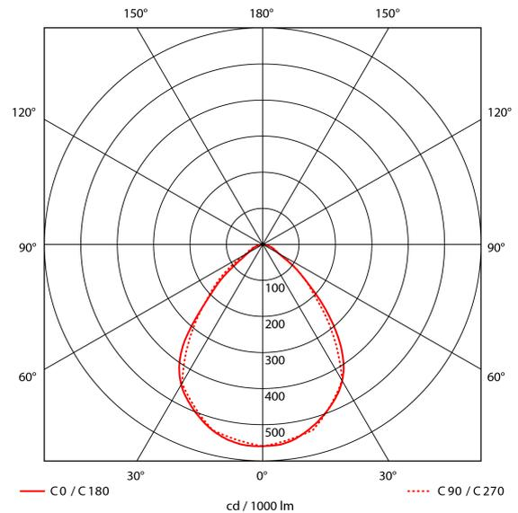
Panel Relax is a luminaire suitable for interior use. Ideal replacement for traditional 3x24W HO T5 and 3x18W T8 fluorescent louver luminaires and side lit LED panel light. Panel Relax have low glare and comfortable light. Comes with a switch option between 3000K(default), 4000K and 5700K. All data is based on 4000K.
