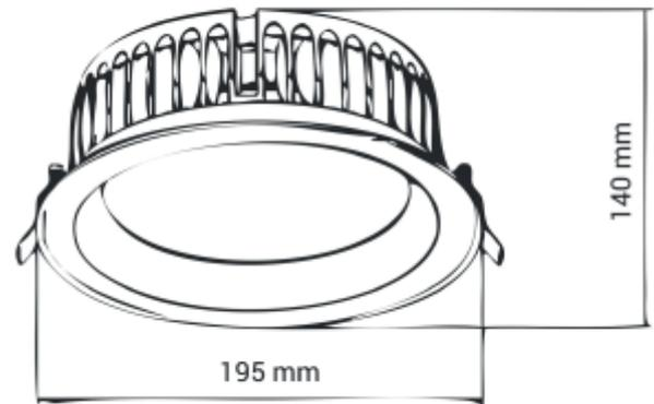
This series of IP44 downlights is named Auriga. Auriga is supplied with 2m cable for power connection.
