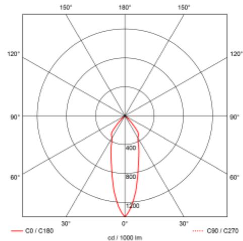
Tigrus 360° Rotatable can be mounted directly in insulation. Downlight have CRI>95 and are delivered with 2700K or Dim2Warm. The downlight can be tilted 25° and it's 360° rotatable. The luminaire connects easily without using a screwdriver. Cut-out 80-83mm.
