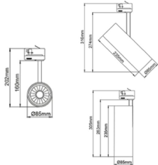
Silindir Maxi is the most powerful spotlight in the Silindir-series. With 28W, high light output and CRI it is very suitable for stores and showrooms. The spotlight can be adjusted in all angles to meet every need. Tilttable 90° and 350° rotatable around its own axis. L305mm - Ø85mm
