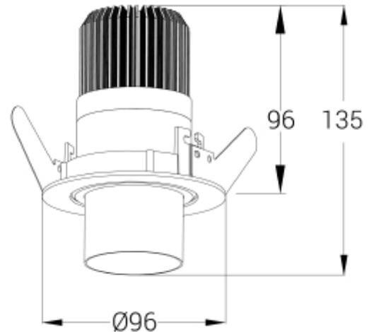
Zoom Recessed, is relatively small downlight with a cut-out size of Ø81mm. The unique zoom patent makes it possible to vary the beam angel between 5 - and 60 degrees making this model highly versatile. The Zoom Recessed is available in both 2700 and 3000 Kelvin and is made from robust die-cast aluminum. Tilttable 25° Please see the table for technical details.
