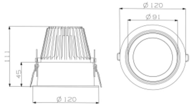
Our Trimo range of downlights guarantees a minimum of stray light. This is accomplished by using a recessed LED light source. This model requires a hole dimension of 112mm in diameter making it very versatile providing very powerful light. The Trimo Mini has a 18i3 connector and is supplied with a variety of connector solutions.
