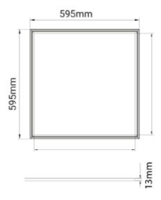
**SPECIFICATIONS** Lightsource Type: LED (built in) System Power [W]: 40W CCT (Color Temperature): 4000K CRI / Ra: 90 Lumen Output: 3138lm Lumen LED (tc=25): 4800lm Lens (Diffuser): Opal Dimming: None System Voltage [V]: 230V 50Hz Connection: IP65 Plug Mounting: Recessed, Ceiling Lifetime [h]: L80B10: 100 000h Color: White Length [mm]: 595mm Height [mm]: Width [mm]: 595mm
