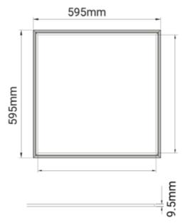
LED Panel with black frame and micro prismatic diffuser.
