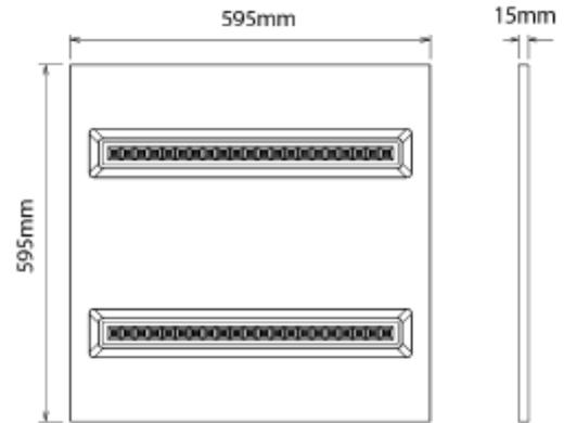
Panel Relax is a luminaire suitable for interior use. Ideal replacement for traditional 3x24W HO T5 and 3x18W T8 fluorescent louver luminaires and side lit LED panel light. Panel Relax have low glare and comfortable light. Comes with a switch option between 3000K(default), 4000K and 5700K. All data is based on 4000K.
