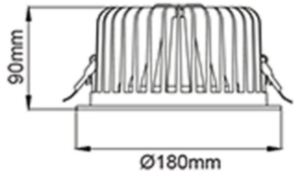
Leila C Midi is a highly efficient downlight with 126 lm/W. With wide beam angle and rotationally symmetric light distribution, it's suitable for all places that require high lumen output. Can be delivered with on / off, phasecut or DALI2 driver. See accessories for suitable driver.
