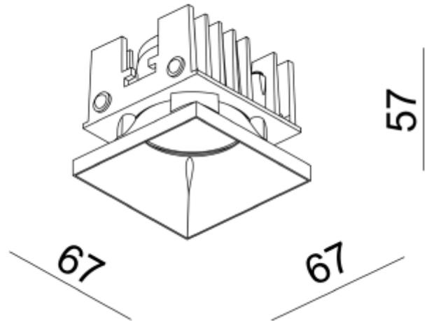
Square downlight suitable for most rooms. Single and double installation kit must be bought separately.
