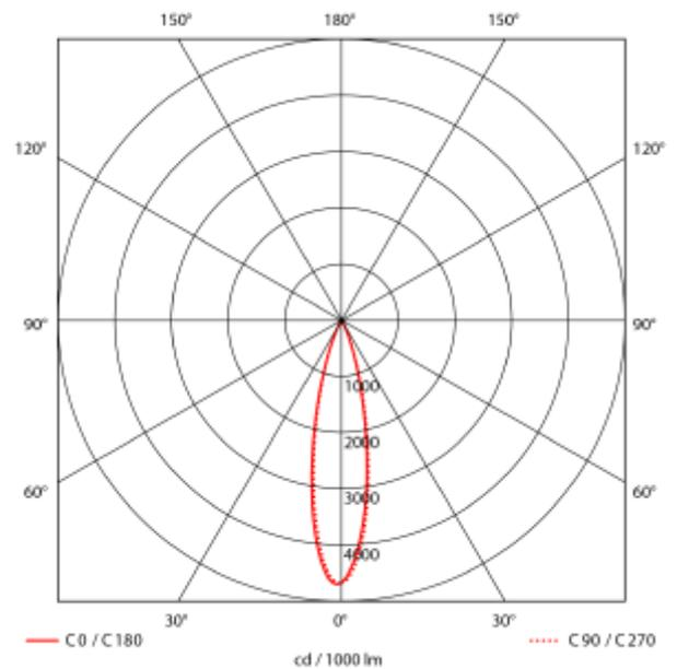
Flare26 is a spotlight that fits our Evo 48V Track system. With 2W, high lumen output, this is a spotlight perfect for housing, stores, restaurants, hotels and office environments. The spotlights can be adjusted in all angles to fit every need. Can be tilted 90 degrees and 350 degrees rotatable around its own axis.
