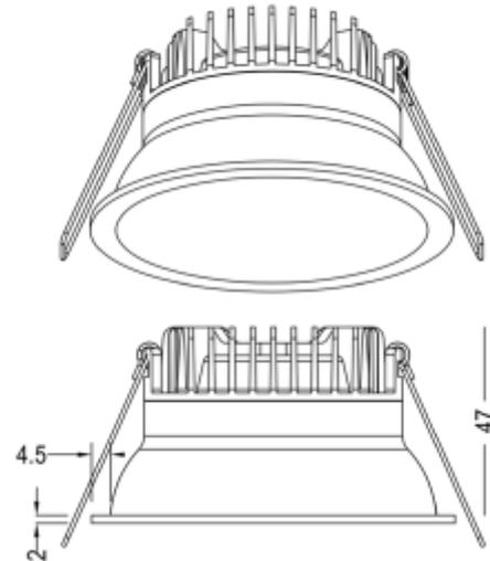
Ceto Mini fixed is a low downlight with 7W effect. With recessed light source, low blending, CRI95 and 18° beam angle, this is the natural choice where you want to create an exclusive and comfortable lighting. Phase-cut driver included.
