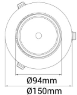
Seta Mini is a small and very flexible LED downlight offering great number of adjustment possibilities. The Seta Mini is supplied with a cable connector type 18i3- and can be delivered with a variety of connector options. The downlight is available in three different colors and with a wide range of reflectors. Rotatable 350° and tiltable 70°.
