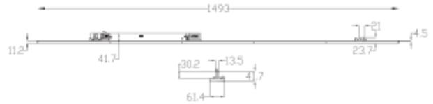
T-Line is our new luminaire for mounting directly into 3-phase track. By using DIP-switch on the wattage setting, you can adjust power to optimize your wattage setting. Choose between 35/40/45W. Preset is set at 50W. T-line comes in 3000K or 4000K with 90°, 120° or double asymmetric beam.
