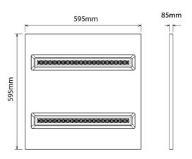
The Relax Par is an interior light fixture designed for recessed installation in suspended ceilings. It is designed with a Louvre front cover in order to achieve less glare and thereby giving a better impression of the light. The Relax Par is equipped with a 18i3 connector and is available in 3 different models, with a variety of connector options.
