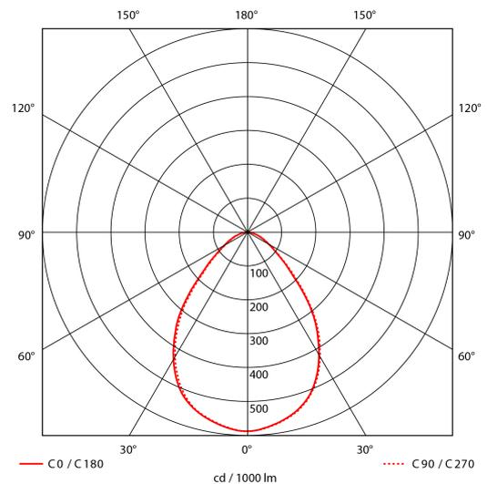
Antares downlight have high lumen output and PMMA diffuser with even light distribution. Choose between opal or microprismatic diffuser. Comes with a switch option between 3000K(default), 4000K and 5700K. All data is based on 4000K.
