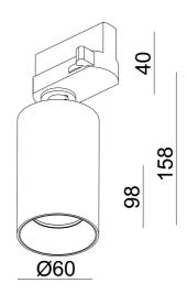
Tania Mini is a small and modern spotlight. Choose between 1- or 3-circut connection. GU10 bulb are not included. Gold front ring can be bought separately. L90mm Ø60mm (GU10).
