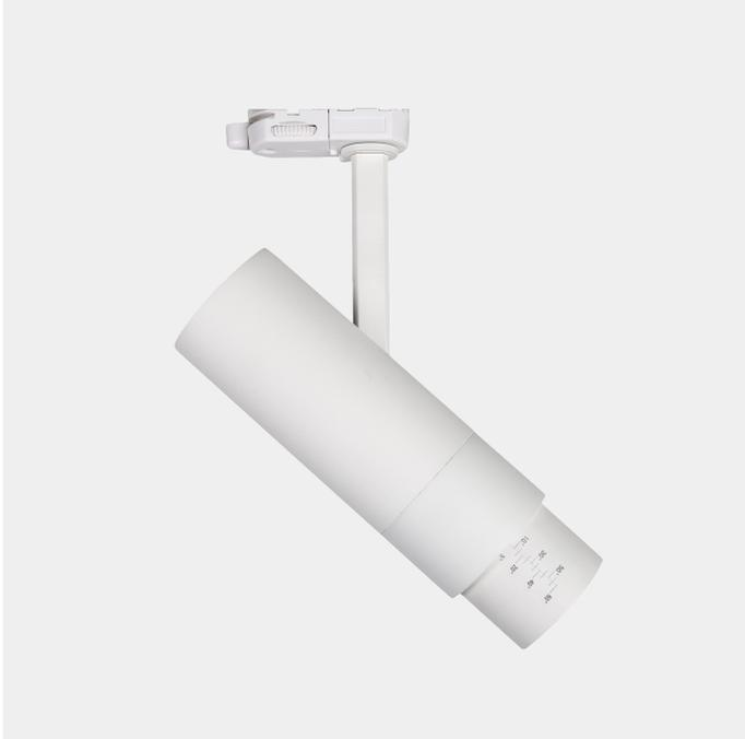
The unique zoom patent makes it possible to vary the beam angle between 6 - and 60 degrees making this model highly versatile. Dimmable by knob on top of the spotlight. The Zoom is made from robust die-cast aluminum.
