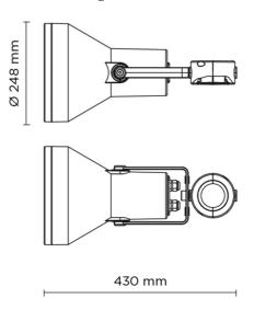
Round pole-mounted floodlight designed for outdoor installation on a pole with a diameter of either 60 mm. The body is made of phospho-chromatised and polyester powder-coated die-cast copper-free aluminum, featuring tempered safety glass, a molded silicone gasket, and stainless steel screws. A clamp for poles with a diameter of 60 mm is included. It comes with a built-in LED driver operating at 220-240V, 50-60Hz, equipped with 1 CREE CXB 3070 COB LED. The floodlight has an IP65 rating.
