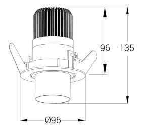
Zoom Recessed, is relatively small downlight with a cut-out size of Ø81mm. The unique zoom patent makes it possible to vary the beam angel between 5 - and 60 degrees making this model highly versatile. The Zoom Recessed is available in both 2700 and 3000 Kelvin and is made from robust die-cast aluminum. Tiltable 25° Please see the table for technical details.
