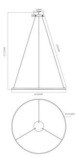
The Halo pendant range consists of 3 different sizes circular luminaires, they are made from aluminum, coated with a golden matt color. The opal surface covering the LEDs gives a very pleasant warm light in 3000 Kelvin. The length of the wires holding the circular luminaires can be adjusted on site making the Halo pendant very flexible for decorative purposes (wire length is 200cm).
