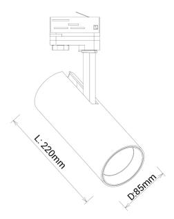
The Cylinder uses the possibilities created by new technology. The LED driver is mounted inside the luminare body. This gives us a slim design combined with a powerful light output that can be easily adjusted in all directions to meet all needs. Cylinder can be tilted 90 degrees and rotated 350 degrees its own axis. To create further opportunities to "play" with light you can mount a diffuser on the luminaire, this can be ordered separately.
