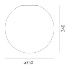
Materials: Thermoplastic resin ceiling support; acid-etched blown glass diffuser. IP65 rating makes it suitable also for outdoor use. (Only for 25, 35, 42 versions)
