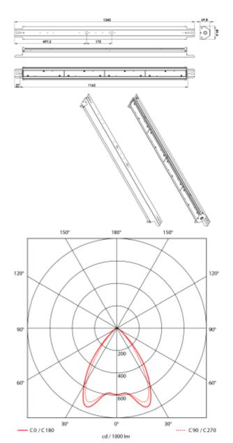
Bladeline Z is a highly efficient LED luminare with up to 179lm/w. Due to fact that it may be installed surface mounted on the ceiling or on electrical tracks makes it highly flexible. Can be opened without using tools and it has the electric connectors on quick fit clamps. The Bladeline Z is made from galvanized steel with medium or wide beam (75° and 90°) optic in 42W or 75W versions.
