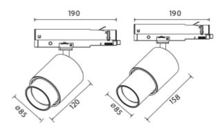
The unique zoom patent makes it possible to vary the beam angel between 6 and 60 degrees making this model highly versatile. The Zoom is available in both black and white versions and is made from robust die-cast aluminum.
