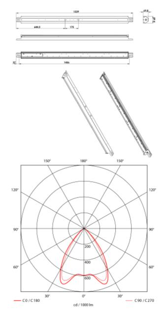
Bladeline Z is a highly efficient LED luminare with up to 179lm/w. Due to fact that it may be installed surface mounted on the ceiling or on electrical tracks makes it highly flexible. Delivered with quickconnect and strain relief in borth ends.
