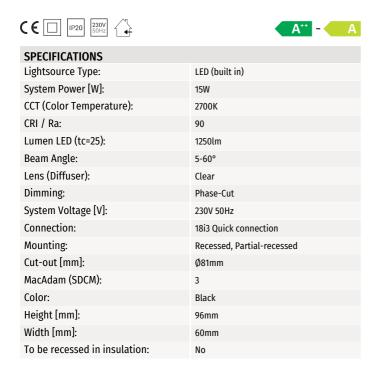
Zoom Recessed, is relatively small downlight with a cut-out size of Ø81mm. The unique zoom patent makes it possible to vary the beam angel between 5 - and 60 degrees making this model highly versatile. The Zoom Recessed is available in both 2700 and 3000 Kelvin and is made from robust die-cast aluminum. Tiltable 25° Please see the table for technical details.
