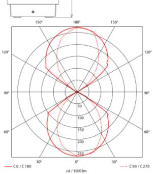
Outdoor luminaire with a modern design with up and down light. Beam angles are adjustable from 15°-210° by changing position of flaps. Made of die-cast aluminum.
